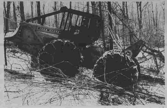
A cable skidder, above, drags logs of any length out of the woods, where they are cut into the desired lengths. The machine is best
